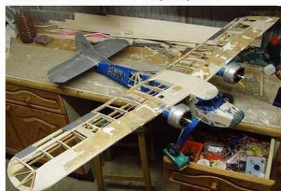
**Step 3:** Admire the result before covering – and risking a test flight.
